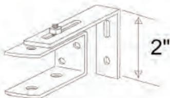
Extension brackets require a 2" flat surface for mounting.
